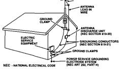
information with respect to proper grounding of the mast and supporting structure, grounding of the lead-in wire to an antenna discharge unit, size of grounding conductors, location of antenna discharge unit, connection to grounding electrodes and requirements for the grounding electrode.
