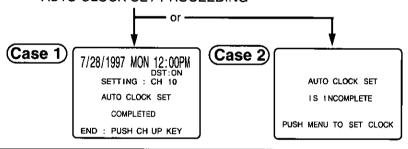
(Case 1) Confirm that displayed time is correct and push A to exit.
